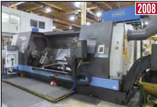
DOOSAN Puma Model 700L CNC Turning Center
