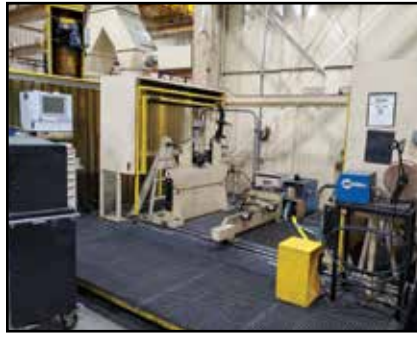
HOFMANN Balancing Stand w/Approx. 7' x 10' Capacity
