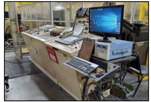
60-HP Dynamometer Motor Test Stand AC/DC #5
