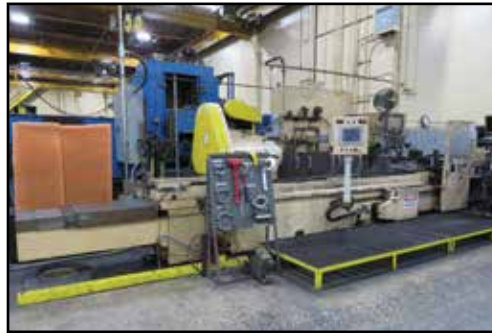
LANDIS Cylindrical Grinder w/Approx. 26" x 145" Capacity
