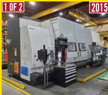
OKUMA LB45III Large Capacity CNC Turning Centers with Y-Axis & Milling
