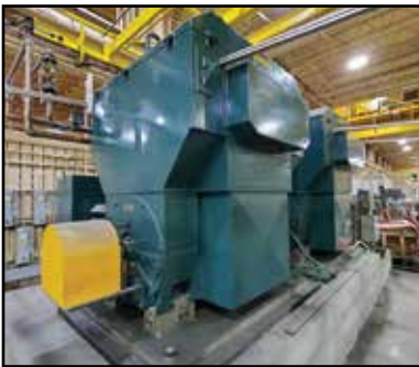
2,500-HP Dynamometer Dual Motor Test Stand
