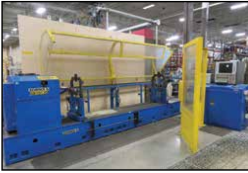
SCHENK BRU 0002 Armature Balancing Machine
