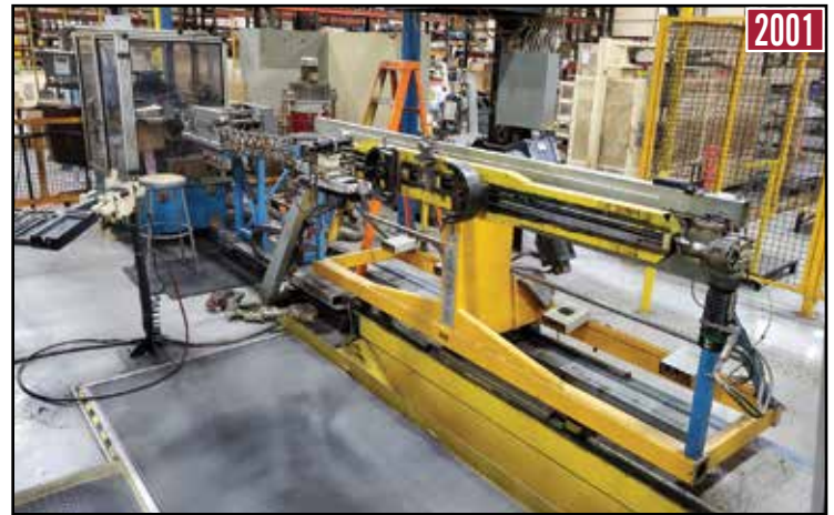
SPIREX Spirex Wind Automatic Tape Winding System
