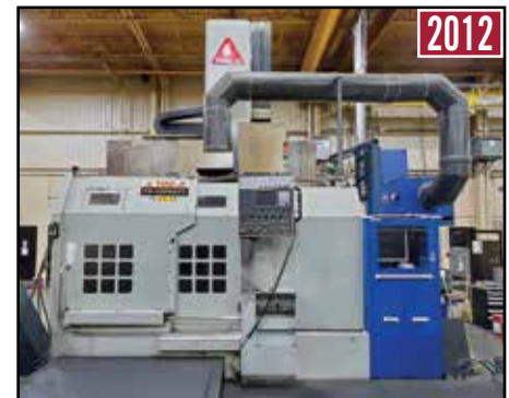
YOU JI YU-1200ATC CNC Vertical Turret Lathe
