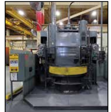
BULLARD 46" Vertical Boring Mill
