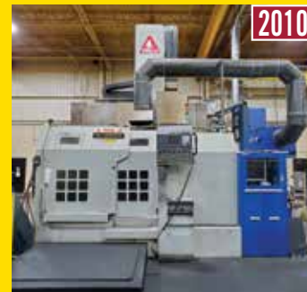
YUJII YV-1200ATC 47" CNC Vertical Boring Mill
