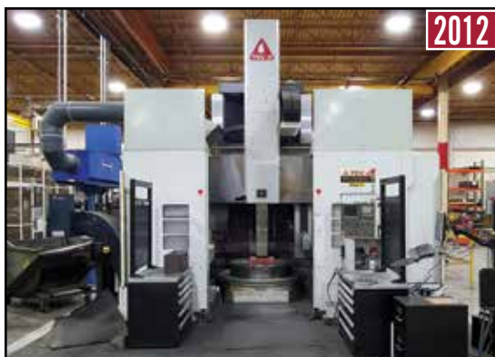
YOU JI VTL-1200ATC-II CNC Vertical Turret Lathe
