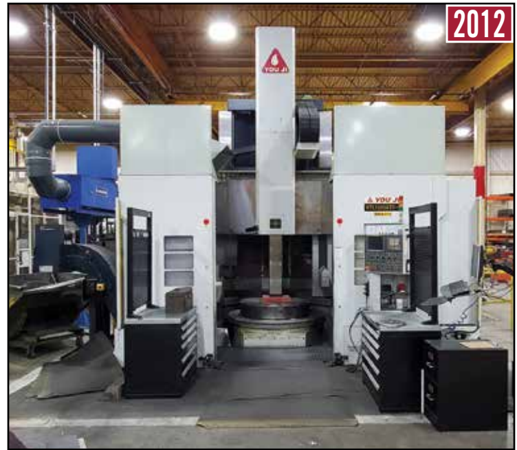
YOU JI VTL-1200ATC-II CNC Vertical Turret Lathe
