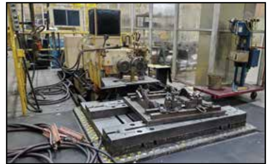
500-HP Dynamometer Motor Test Stand
